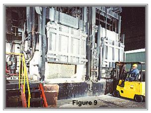
Aluminum is tapped and then pumped to the caster from this well during casting cycles. Metal is also circulated through this well, through a scrap charging well, and to the charging area of the melting chamber.
