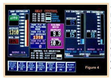
This display is used to set the bath temperature desired and also indicates the air/gas ratio of the burners (Figure 4). The bath temperature is controlled by changing the burner operation mode. There are four modes of burner operation used during the charging/casting cycle:
