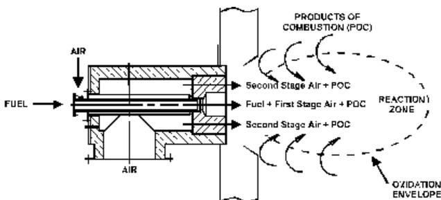
Figure 1: LumiFlame Ultra Low NO<sub>x</sub> Concept
