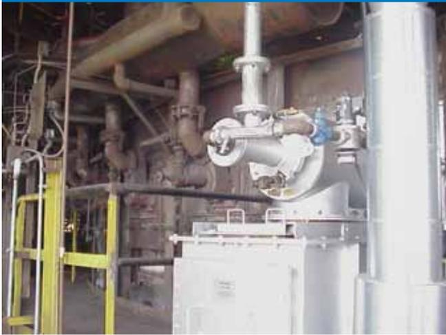
Hybrid retrofitted regenerative cold air furnace.
