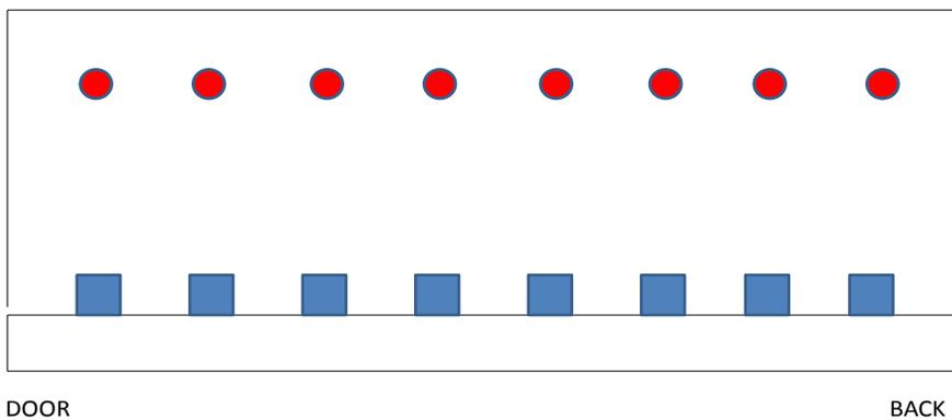
The following is the fuel distribution for the batch furnace:
