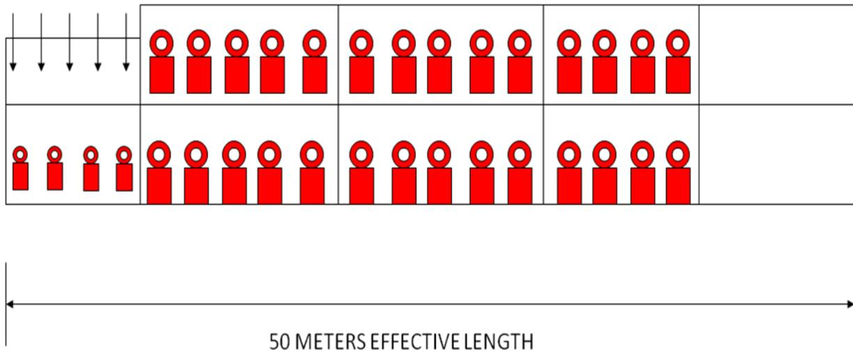
The furnace yielded a fuel rate of 243 Kcal/Kg at the design tonnage. Other relevant performance criteria were 30-55 ppm NO<sub>x</sub> at 12% O<sub>2</sub>, 0.33-0.54% scale loss, and 18°C head to tail differential. All of these values exceeded the performance criteria.
