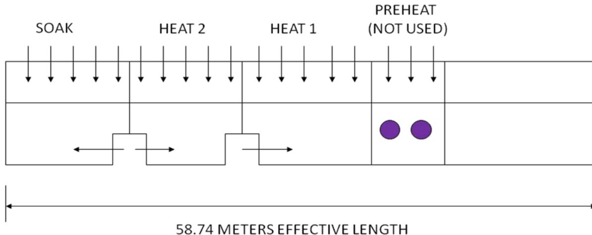
The doghouses were removed and regenerative burners were installed in the bottom heat 1 and heat 2 zones. The following is a schematic diagram of the furnace after it was modified.
