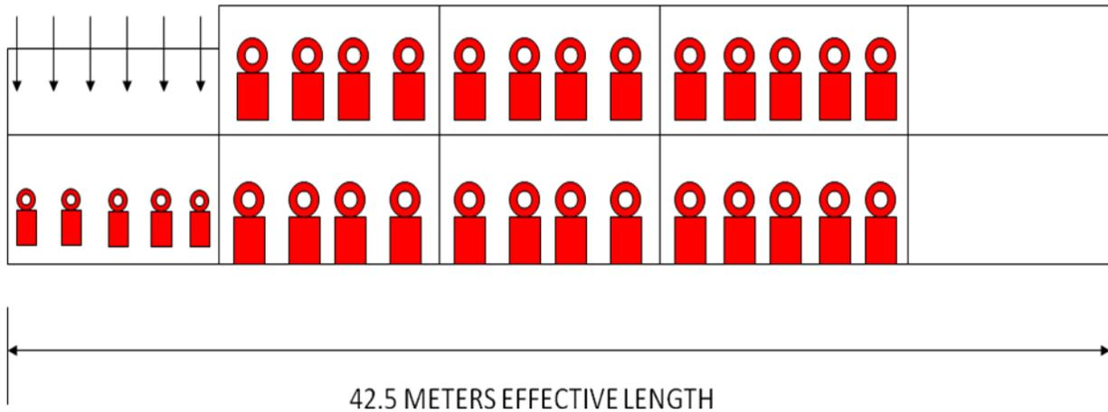
The furnace yielded a fuel rate of 262 Kcal/Kg at the design tonnage. Other relevant performance criteria were 30-55 ppm NO<sub>x</sub> at 12% O<sub>2</sub>, 0.33-0.54% scale loss, and 18°C head to tail differential. All of these values exceeded the performance criteria.
