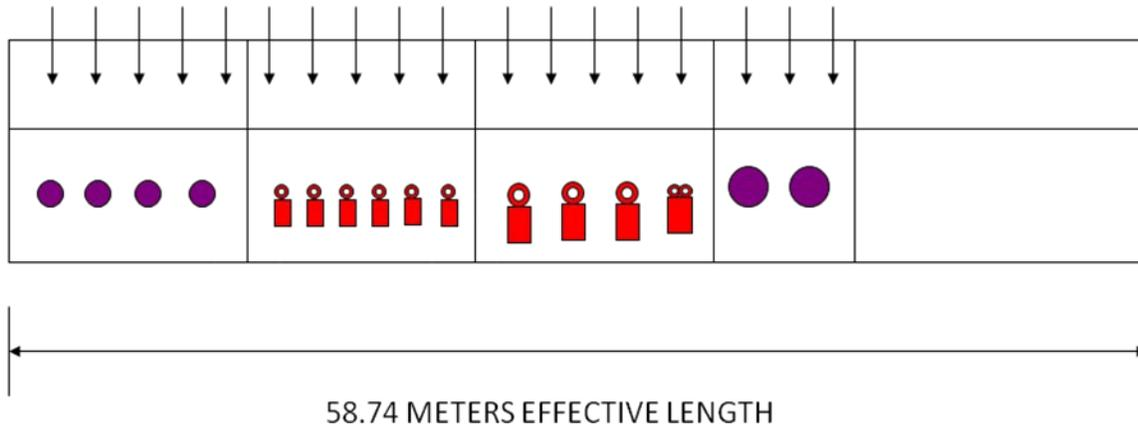
The modified furnace yielded a 9.6-18.8% fuel savings. The guarantee value was 8.2% at full production. Other relevant performance values were 47 ppm NO<sub>x</sub> at 11% O<sub>2</sub>, 1120°C air preheat at the burner head and 140°C exhaust gas temperature. All of these values exceeded the performance criteria.
