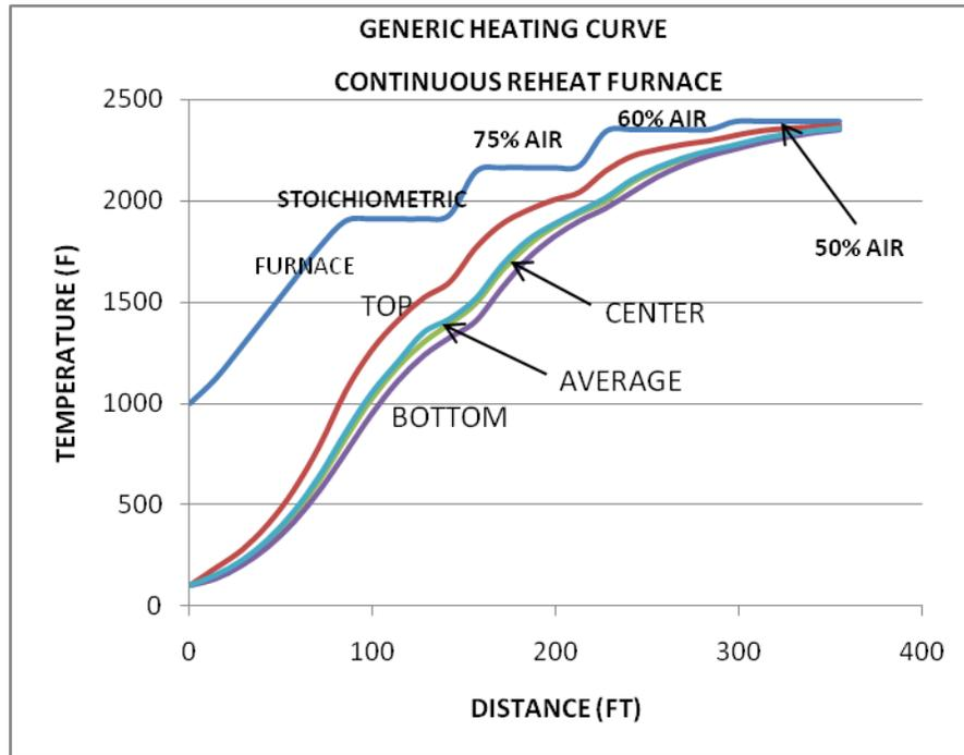
Temperature/Combustion Profile of a Continuous Furnace
