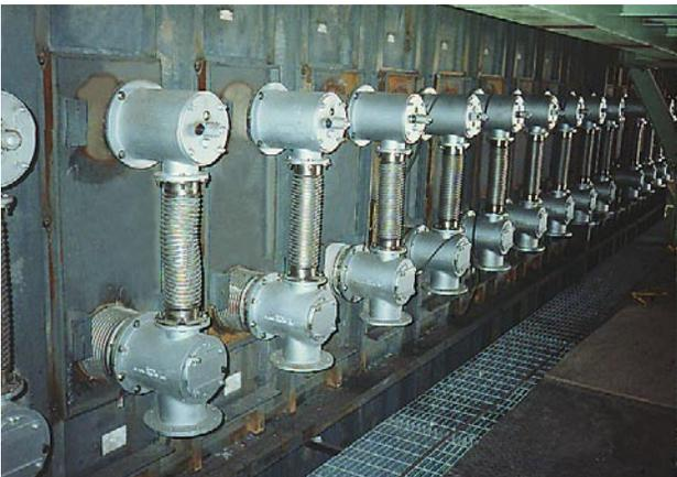
Vertical Strip-heating furnace with radiant 'W'-tubes
