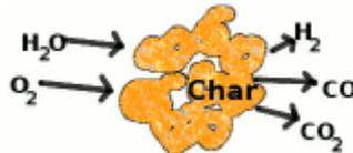
The high costs of capital equipment including extensive flue gas cleanup has limited the feasibility of such projects. However, a future optimized technology can be envisioned in which oxygen-blown coal (or biomass) gasification would yield a gaseous fuel with primarily H<sub>2</sub> and CO<sub>2</sub> combustion products. This would then minimize the difficulty and expense of carbon sequestration.
