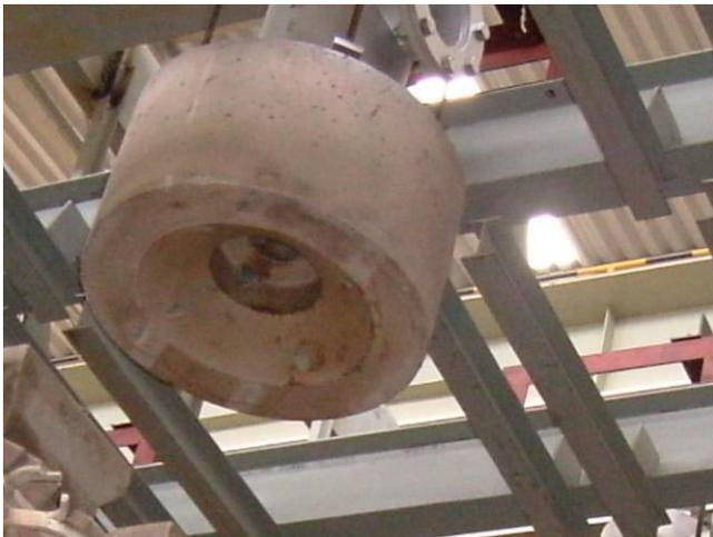
Roof-mounted flat profile flame burner
