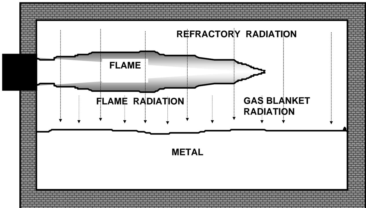
In an aluminum holding furnace, the area of the receiver is limited to square footage of bath surface. The ability of the surface area to absorb heat is complicated by the dross formed on the surface. A thin layer being preferable to a shiny reflective surface.
