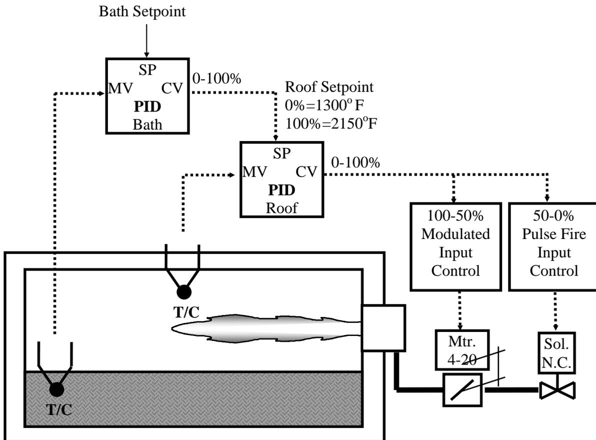
Control Loop 1 - monitors the metal bath temperature and varies the 4-20ma output based on the difference between the bath temperature and the set point. If the metal is at or above set point, the output is 4ma. If the bath temperature decreases, the output increases to a maximum of 20 ma is necessary.
