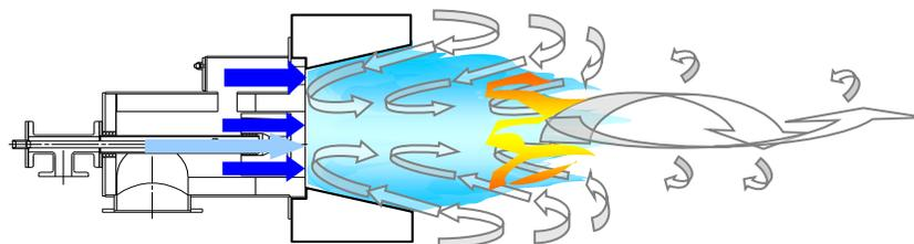
Picture 8 – Bloom 1440 Series Burner Principle
