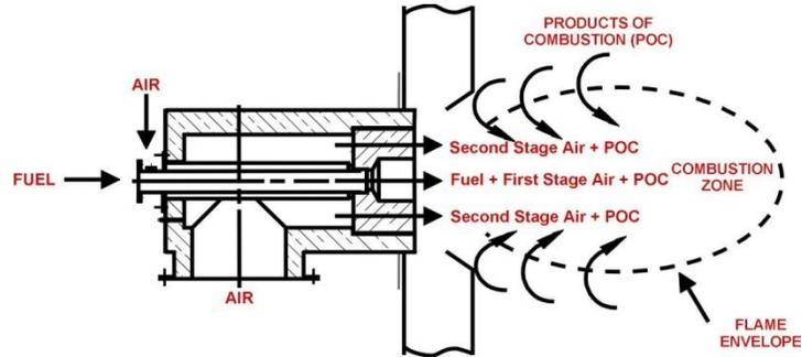
Figure 1 – Bloom Baffle Burner Design
